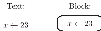
Figure 4.1: An assignment operation in both text language (left), and block language (right).
